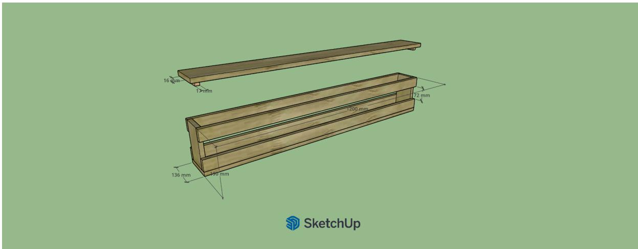
**Technical Note:** To ensure the lid is secure and does not shake or open easily, you must attach **fixing bars** to the underside of the lid. These bars should precisely match the **upper inner diameter** of the feeder body on both sides for a snug fit.
