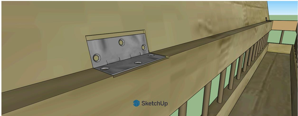
**Technical Note:** For the lid to close perfectly and remain flush with the body, the area where the **hinges** are attached must be **slightly recessed (mortised)**. Carving out a small amount of wood in these spots is essential for a professional, seamless finish.
