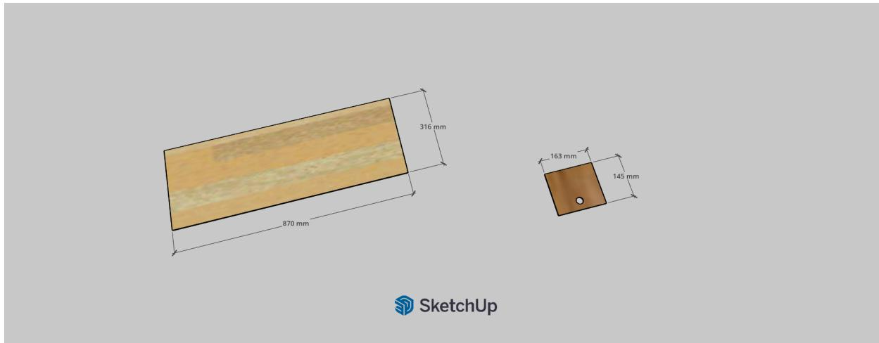
**Technical Note:** Specifications for the removable waste tray (bottom) and the small entry door (top) used for loading pigeons. These parts are designed to slide or fit precisely within the main frame dimensions.
