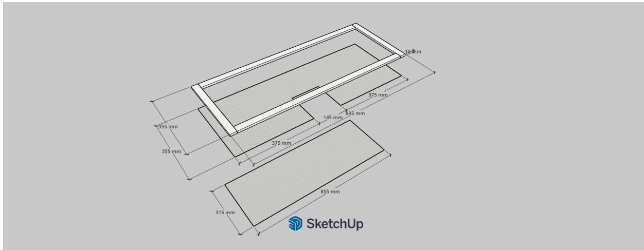
**Technical Note:** Detailed dimensions for the top wire mesh, the frame-style retainer strips (cleats) that secure the mesh from above, and the bottom floor mesh. Accurate cutting of the retainer strips ensures the mesh remains taut and secure.
