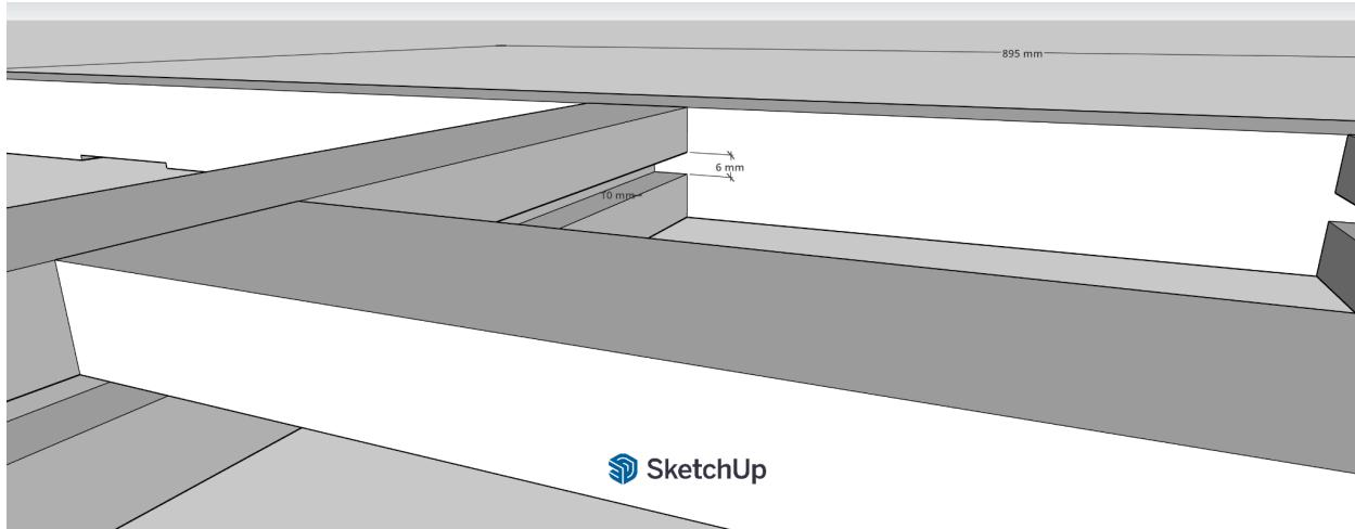
**Technical Note:** Close-up view of the top entry door's frame grooves. Like the bottom tray, these require precise grooving with a **Table Saw** or **Trimmer**. Refer to the marked height and depth to ensure the top door slides smoothly without jamming.
