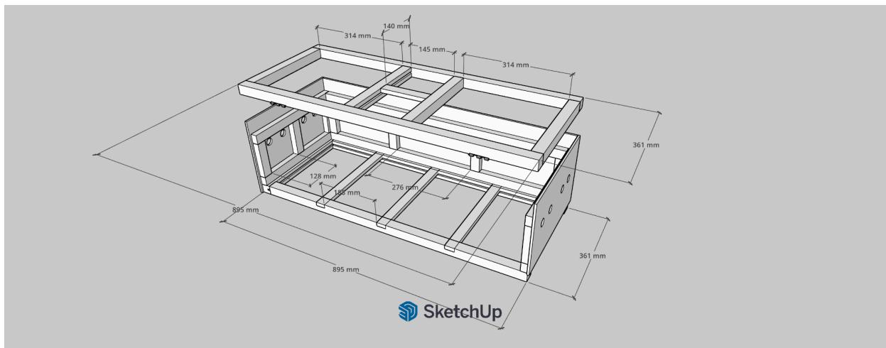
**Technical Note:** This image shows the core structure, including both side panels, the back panel, and the bottom/top frames. Key lengths and widths are marked for the basic skeletal assembly. Ensure all frame connections are square to maintain structural integrity.
