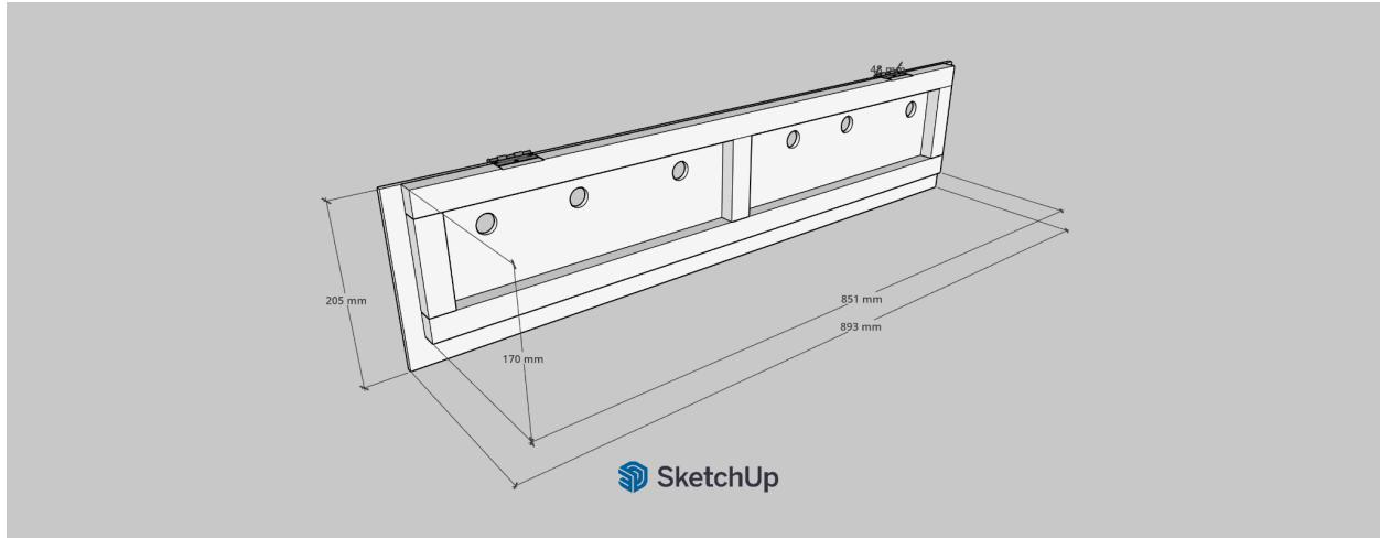
**Technical Note:** The front door is designed with a top-hinge system that opens from bottom to top. **Note:** The internal frame height is intentionally 1cm shorter to prevent interference when opening. However, the 6mm front plywood covers the entire front face for a seamless and clean exterior aesthetic.
