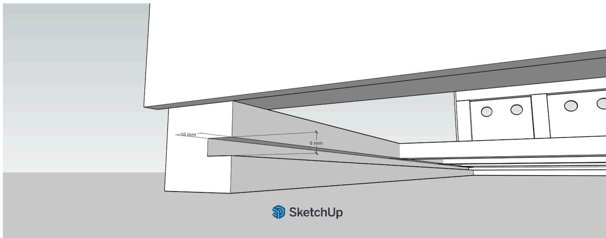
**Technical Note:** Close-up view of the bottom frame grooves. These grooves serve as rails for the waste tray and must be carved using a **Table Saw** or **Trimmer**. Detailed measurements for the groove height and depth are provided for precise sliding action.
